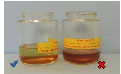
**Figura 2. Nível do óleo**
